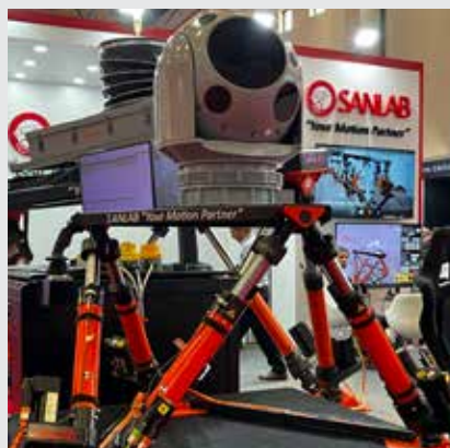
Electro-Optical System Test Application
