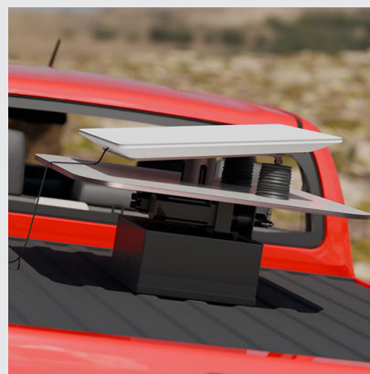
Land Vehicle Antenna Stabilization Application
